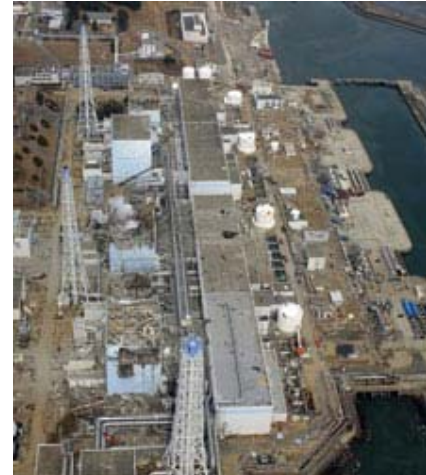
Figure 2. Aftermath of Fukushima Daiichi accident on March 18, 2011, one week after the accident. Rubble from hydrogen explosions in units 1, 3 and 4 is spread over the site. Damage from the earthquake and tsunami to the electrical systems is apparent along the water front. Steam still emanating from unit 2. Source: DigitalGlobe
